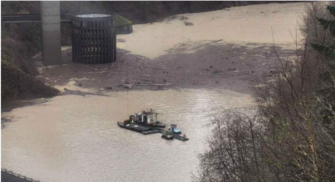
Photo 7-2. MMD Log Broncs and Work Boat at Dock Ready for Deployment at High Reservoir Inundation Elevation
