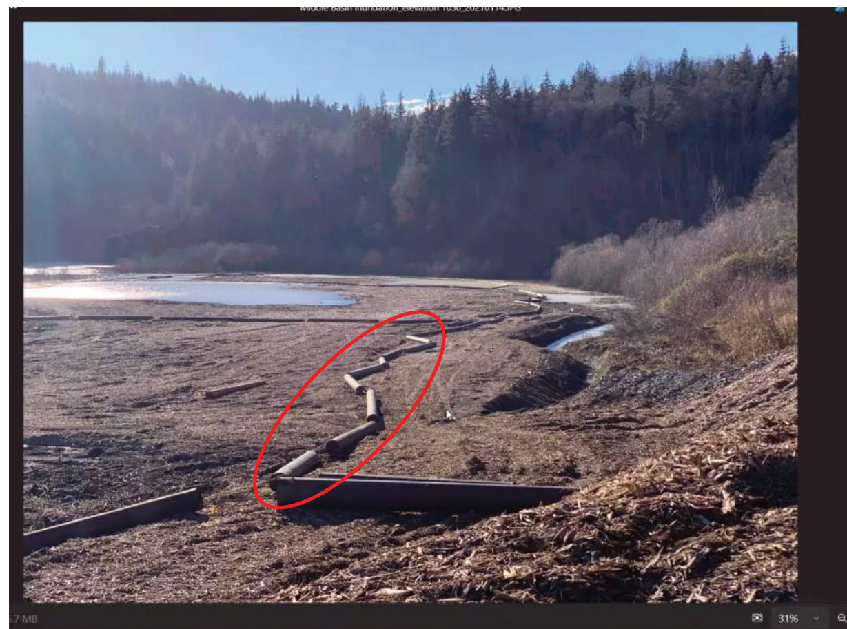
Image of steel boom logs tied end to end – used to encircle one 'sack' and bring to the boat for hauling
