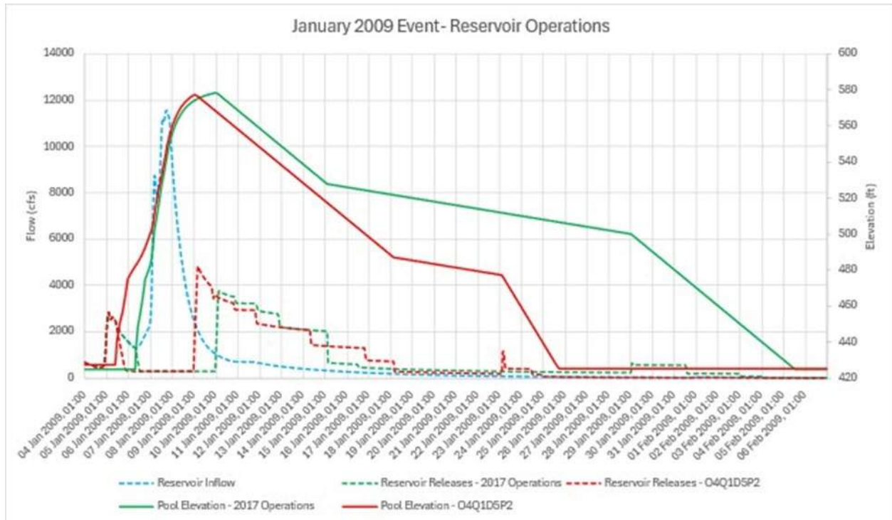
Figure 2. Reservoir Elevations, Inflows, and Releases - 2017 Operations and O4Q1D5P2 Operations
